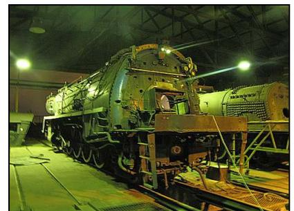
With her boiler backhead crudley exposed after removal of the cab, 15F No.2914 is starting to undergo firebox repairs.
